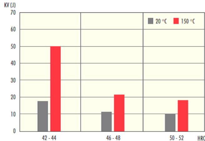
Figure 5. Variation of impact strength with hardness for different working temperatures [1]
