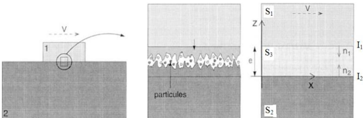
Figure.6: system of two bodies in contact and their interfaces [4].
