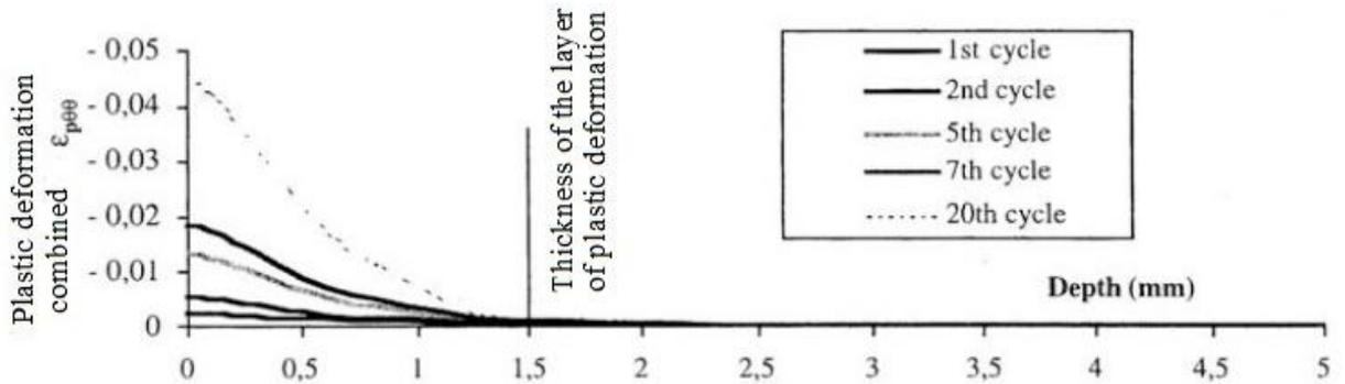
Figure.10: Accumulation of the plastic deformation in function of the number of cycles [14].
