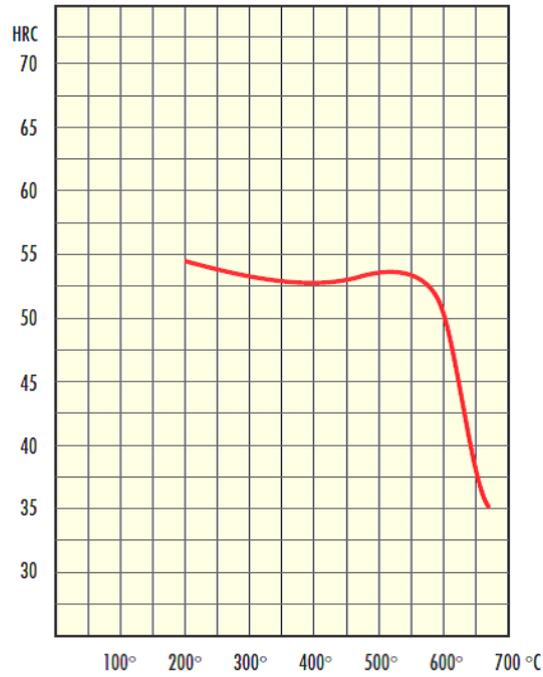
Figure3.Tempering curve (1 cm thick test piece)
