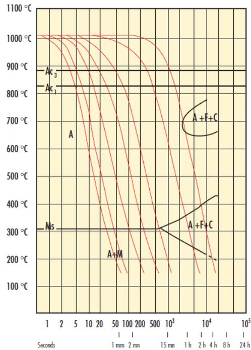
Figure2.CCT diagram Austenitizing at 1010°C
