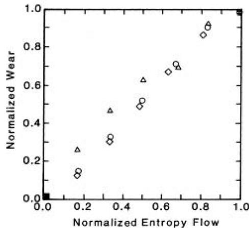
Figure.7: Wear standardized in function of the variation of entropy standardized, each point represents the average of 4 tests [9].
