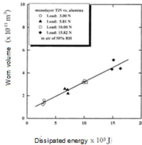
Figure.8: Wear in function of the dissipated energy accumulated in the case of a unidirectional friction of a ball on a disk under different loads [12].
