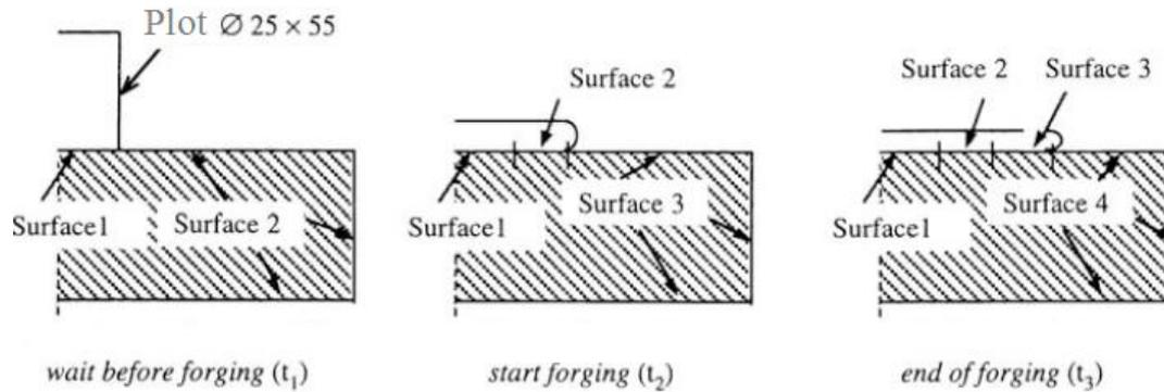
Figure.9: Location of different surfaces taken into account in the identification of thermal flux [14].
