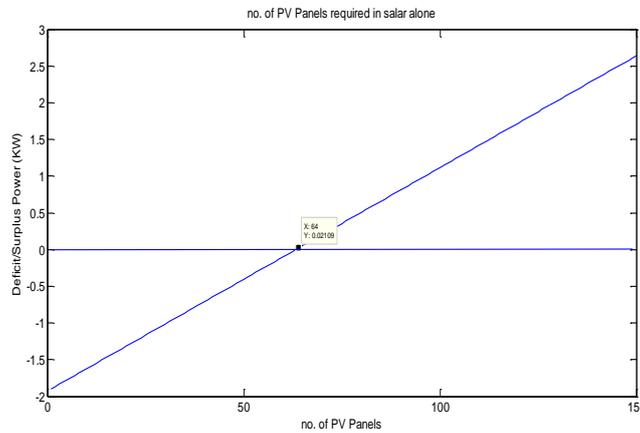
Figure.12. Graph of Deficit/Surplus Power produced by 'n' no. of PV Panels
