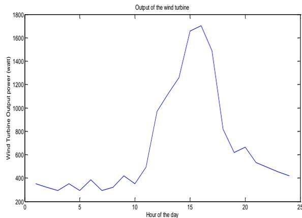
Figure .8 Graph of output of a single wind turbine at each hour of the day
