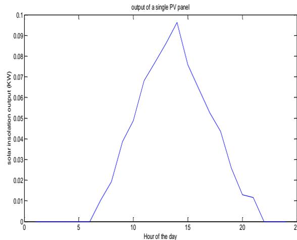
Figure 6 Graph of output of a single PV panel at each hour of the day
