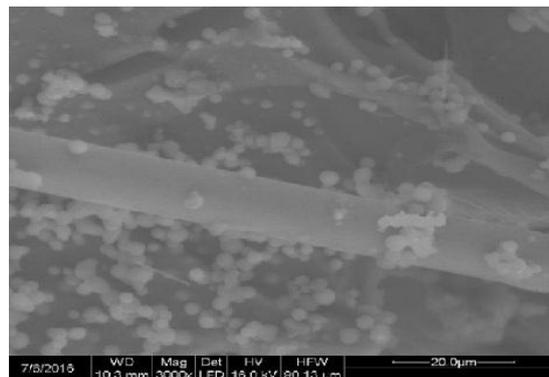
Figure 6. Electron micrographs of a sample degraded for 300 days in 90% H<sub>2</sub>SO<sub>4</sub>
