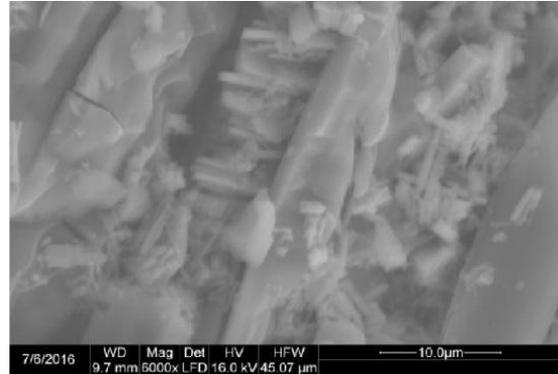
Figure 4. Electron micrographs of a sample degraded for 300 days in 70% H<sub>2</sub>SO<sub>4</sub>
