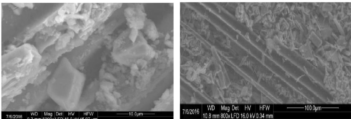
Figure 2. Electron micrographs of a sample degraded for 300 days in 30% H<sub>2</sub>SO<sub>4</sub>
