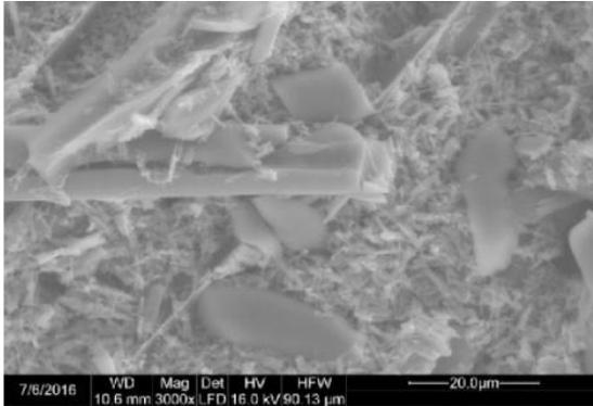
Figure 3. Electron micrographs of a sample degraded for 300 days in 50% H<sub>2</sub>SO<sub>4</sub>
