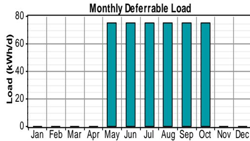
Figure 1. Monthly energy consumption for water pumping
